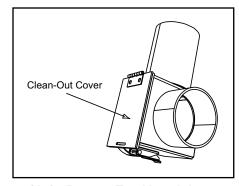
Figure 19.4 - Rear to Top Vent Adapter - 90°
